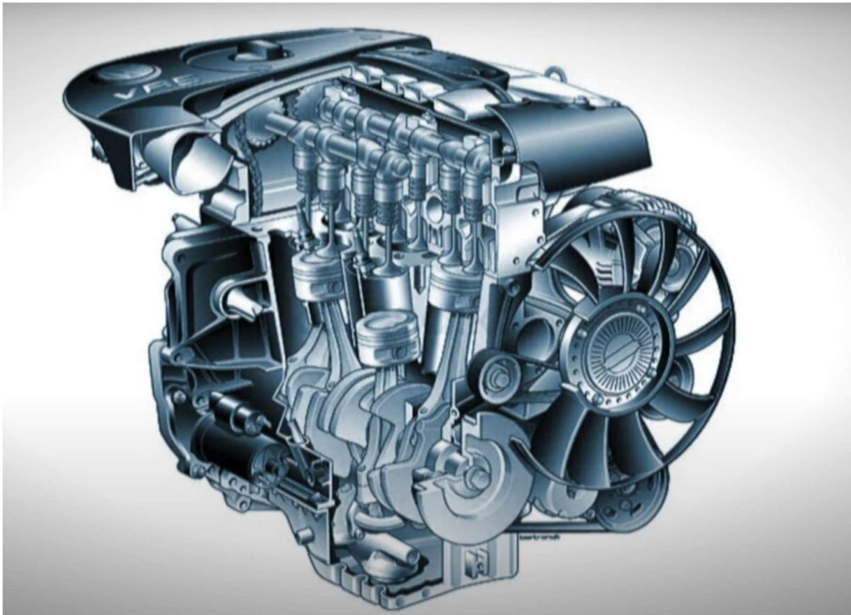
Arguably one of the biggest reasons for VW to pursue the W10 over the W12, was because it would allow each VR5 engine to offset the other's imbalances. The odd firing order within a five-cylinder engine makes it run extremely rough without the addition of balance shafts and whatnot. Photo Credit: VisioRacer/YouTube
